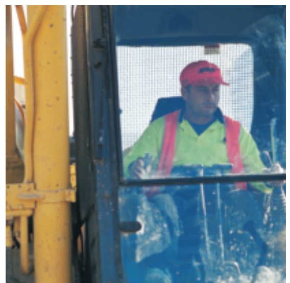
Enclosed cabin to protect operator from noise sources
