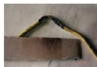
Conditions of PVC and cardboard after 12-13 minutes of exposure
