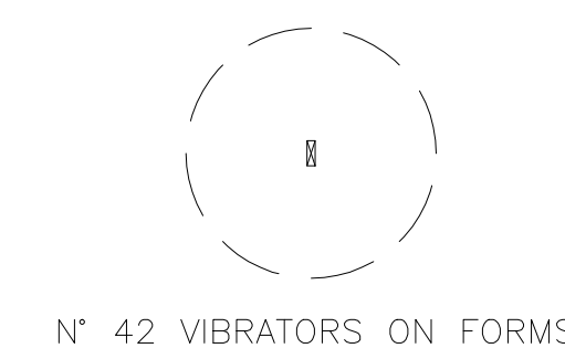
N° 42 VIBRATORS ON FORMS
