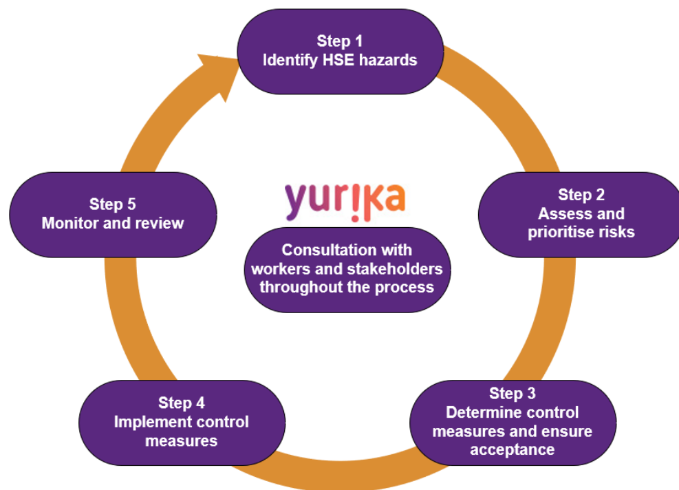
Figure 3 – Five Step Hazard Risk Management Process
