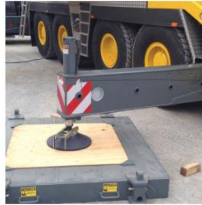
Photograph 3: Bog mat used to spread the applied load.
