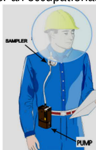
Personal Air monitoring – sampler must be positioned within breathing zone of worker.
