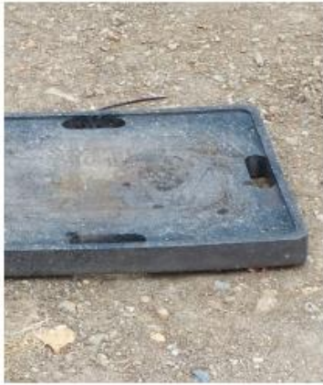
Photograph 1: Outrigger pad on fill with no visual signs that the ground is soft.
