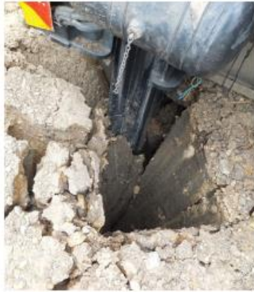
Photograph 2: Outrigger pushed into soft ground after breaking through crust.
