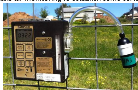
Static Air monitoring – Positioned in fixed locations to determine general exposure levels
