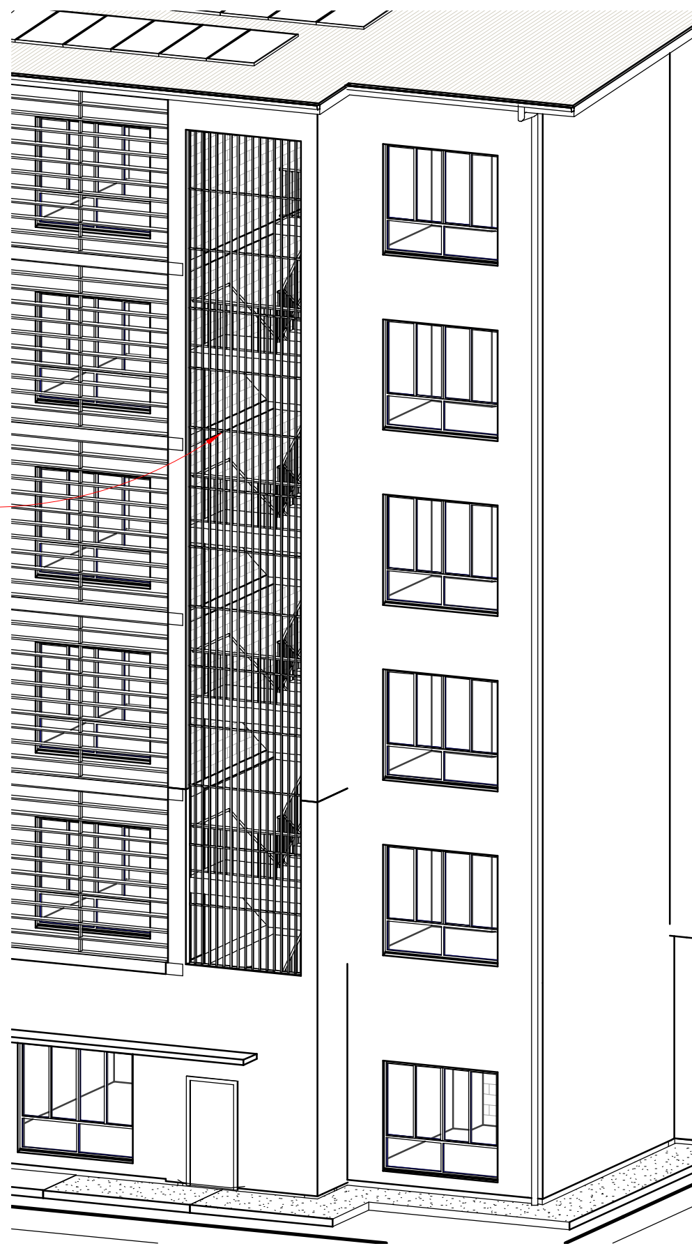
4 Stair 3 - Batten Treatment
