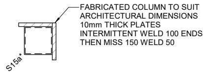
FABRICATED COLUMN S15a* DETAIL SCALE: 1 : 10
