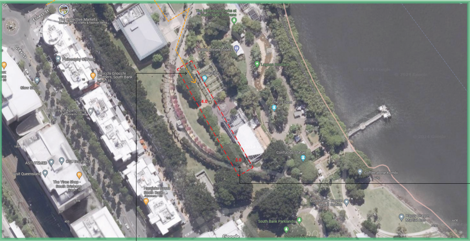
EXTENT OF TREE BASE WORKS. 6 x 1500 x 1500MM BASES.
